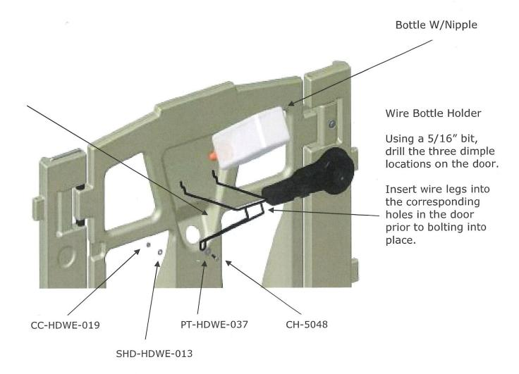
Install the 1" cap screw (CH-5048) and the 1" dia. Washer (PT-HDWE-037) through the bottom loop of the wire bottle holder.
